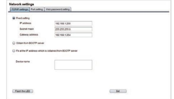
3. Paste the IP address memo label. Write the set IP address on the IP address memo label and paste it on the target reader/writer.
