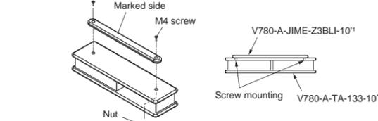
2. Mount the Attachment to which the RF Tag is mounted to the metallic material. Mount it with two M4 bolts. (Recommended tightening torque: 1.2 N·m, M6 bolt mating length: 4 mm min.)
