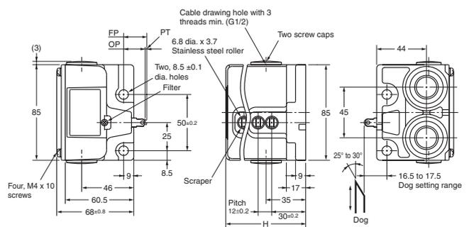
**Note:** Unless otherwise indicated, a tolerance of ±0.4 mm applies to all dimensions.
