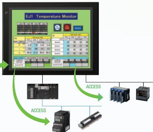
**Support tool objects can be incorporated to check for errors and make settings, even without a computer.**
