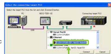
PLCs registered to the PT are automatically searched for. Make the connection simply by selecting from the PLC list.
