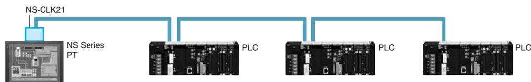
If a Controller Link connection is used, data links can be set between PLCs and multiple PLCs can be monitored/set from the NS-series PT's screen.
