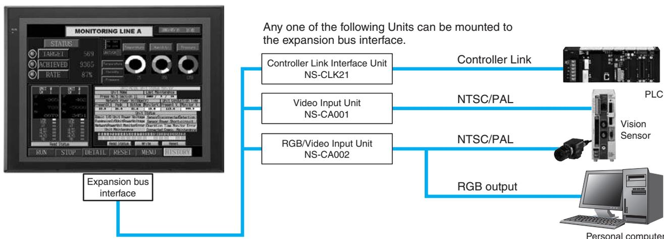
Note: Video Input Units and RGB Video Input Units cannot be used with some models.
