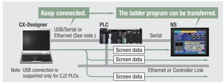
Using a USB relay cable greatly improves debugging at equipment startup.
