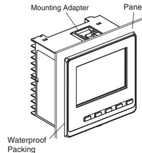
1. In order to make the unit waterproof, with the accessory waterproof packing on the front of the panel, insert the unit into the panel opening.
