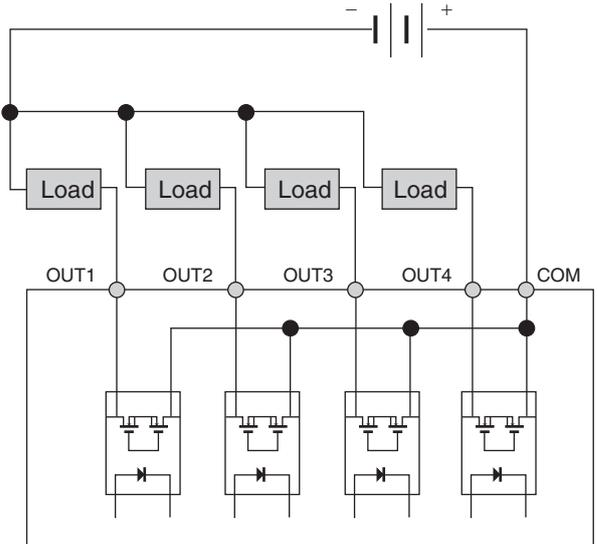
The Power Monitor provides four pulse output terminals. One common is used.
