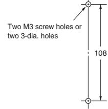
**Note:** Pull out the hooks to mount the Relay with screws.
