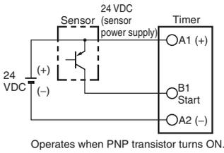
Operates when PNP transistor turns ON.
