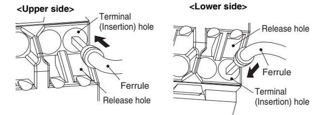
If a wire is difficult to connect because it is too thin, use a flat-blade screwdriver in the same way as when connecting stranded wire.
