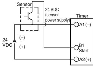
Operates when NPN transistor turns ON.
