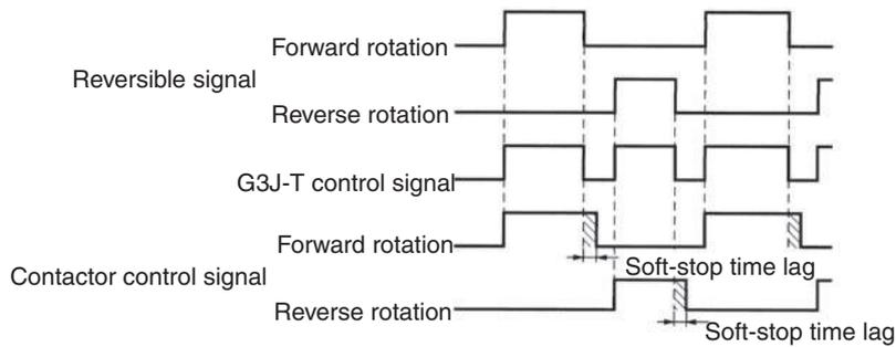
**Note:** Make sure that the interval between forward and reverse operations is at least 100 ms. If the G3J is turned ON by noise input, short-circuiting between phases will result. In order to prevent this, insert a protective resistor.
