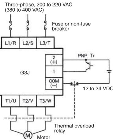
**Note:** 1. When the minimum applicable load of the thermal relay auxiliary contacts becomes smaller than the input current of the G3J, insert a bleeder resistance.
