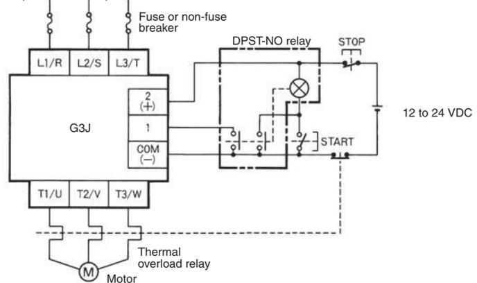
**Note:** Be sure to use a fuse or non-fuse breaker to protect the G3J.
