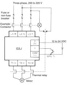
Do not operate motors that exceed the allowable capacity with G3Js connected in parallel. Doing so may result in malfunctions.
