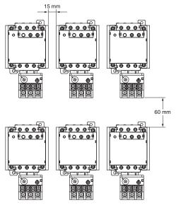
**Note:** Minimum distances of 15 mm horizontally and 60 mm vertically are required between adjacent G3Js with thermal overload relays.
