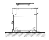
**Note:** When the G3J is mounted horizontally, the load current must be 50% of the rated load current if the G3J is used at a temperature exceeding 40°C.
