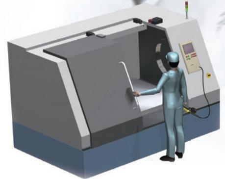
Enabling grip switches are safety components used to prevent unexpected machine operation when workers perform maintenance or other non-routine tasks inside hazardous areas, such as areas inside protective shields.
